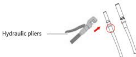
Pic 5.4 Crimp the contact pin to the wire
